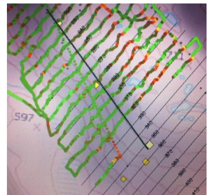
Raw magnetic data plotted while the survey takes place.
