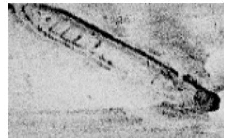
Figure 2: Side scan sonar showing a 30 meter ship wreck.
