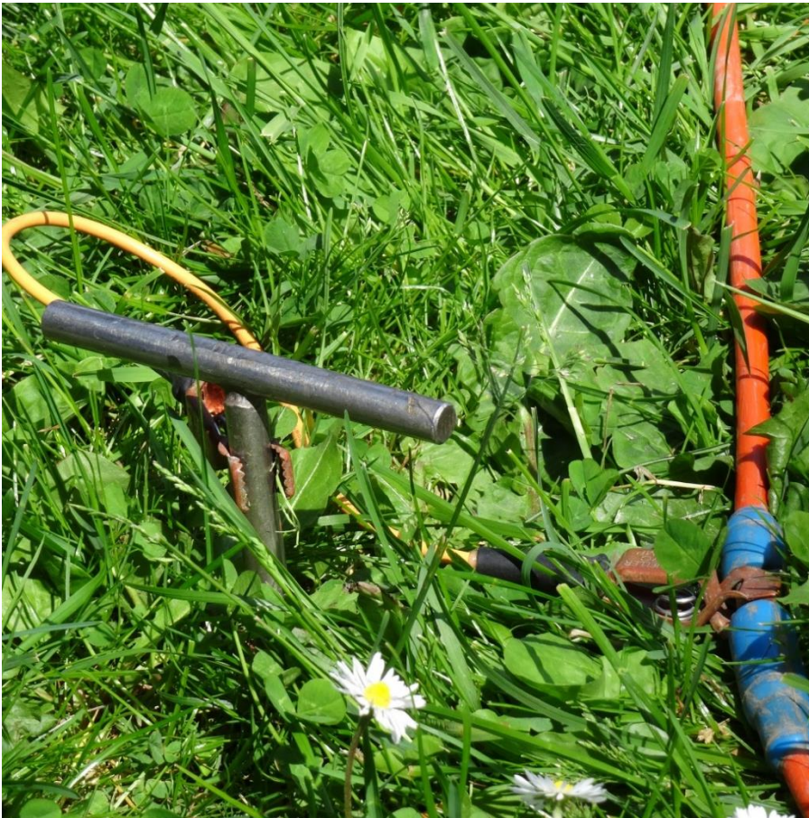
Stainless steel electrode connected to the multicore transmitter and receiver cable
