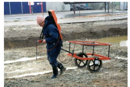
Figure 1: The operator carries a backpack with batteries and a control unit together with a handheld computer.
