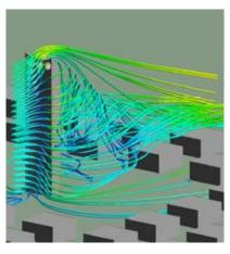
Visualization of CFD results showing the very complex flow patters around a high rise building. The three circular openings at the top of the building will each house one wind turbine and CFD simulations have been used to determine their performance at these unusual operating conditions.
